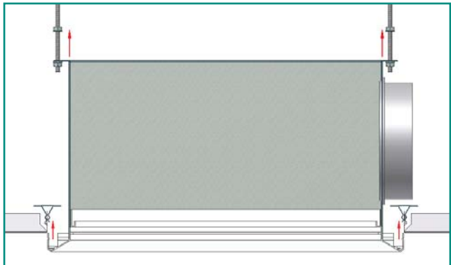
Figure 8: Raise the plenum and diffuser
