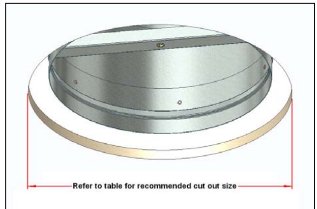
Figure 7: Cut Clearance Hole
