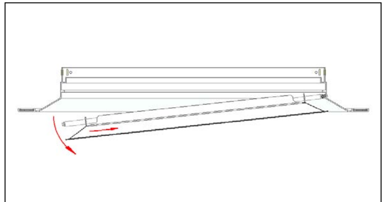
Figure 9: Rotate Core downwards to remove
